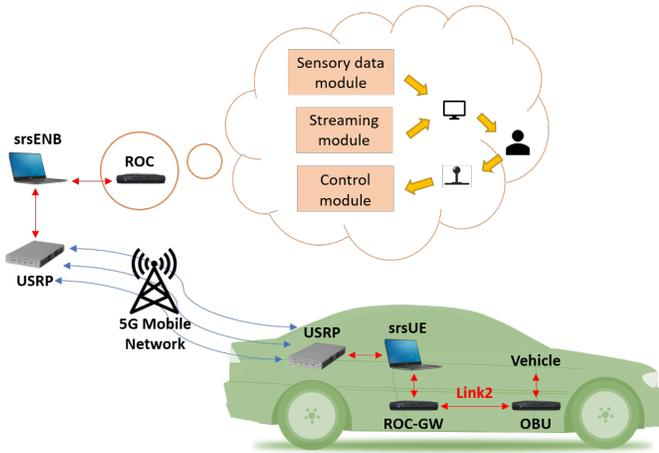
Fig. 1. Overview of the end-to-end architecture of TeSo.
